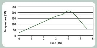
Peak reflow temperature should be <260°C in an air or nitrogen atmosphere (<500ppm  $0_2$ ), with a linear ramp up to 30°C above liquidus temperature. These profiles are recommended to the user as starting points, and should be optimized by the user to meet their individual process needs.
