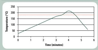
This profile is designed for use with Sn63/Pb37 and Sn62/Pb36/Ag2 and can serve as a general guideline in establishing a reflow profile for use with other alloys. Adjustments to this profile may be necessary based on specific process requirements. Please contact Indium Corporation's Technical Support if you require a reflow profile for a different alloy.
