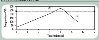
This can be used as a general guideline in establishing a reflow profile (the example above shows the use of Indium8.9HF with Indalloy®292 Solder Paste). Deviations from these recommendations are acceptable, and may be necessary, based on specific process requirements, including board size, thickness, and density. Start with a linear profile. If needed, a flat soak portion or a linear shoulder may be added to reduce the thermal gradient.
