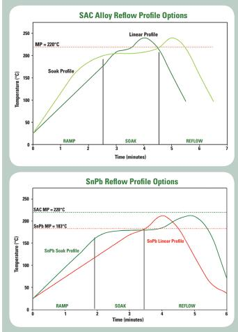
Peak reflow temperature should be <250°C in an air or nitrogen atmosphere, with a linear ramp up to approximately 30°C above the solidus temperature.
