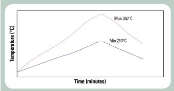
This is the standard reflow profile for 5-SLC. The time to peak should be about 3 to 5 minutes. The peak temperature should be 20°C more than the melting point of the metal. Time above liquidus should be about 40 to 70 seconds.
