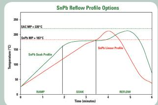
Peak reflow temperature should be  $<250\,^{\circ}$ C in an air or nitrogen atmosphere, with a linear ramp up to approximately  $30\,^{\circ}$ C above the solidus temperature.
