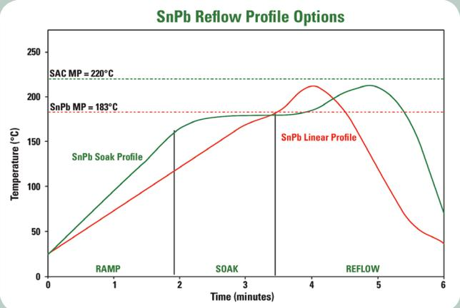
Peak reflow temperature should be <math><250^{\circ}\text{C}</math> in an air or nitrogen atmosphere, with a linear ramp up to approximately
