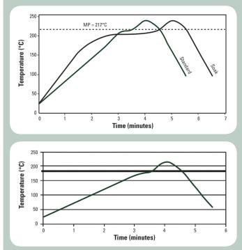
Peak reflow temperature should be <250°C in an air or nitrogen atmosphere, with a linear ramp up to approximately 30°C above the solidus temperature.
