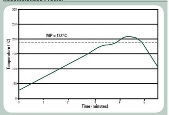
This reflow profile is designed for use with 63Sn/37Pb. Adjustments to the profile may be necessary based on specific process requirements.
