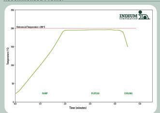
This profile is designed for use with **Durafuse® LT 195**. This can be used as a general guideline in establishing a reflow profile for **Durafuse® LT 195** Solder Paste. Deviations from these recommendations are acceptable, and may be necessary, based on specific process requirements.
