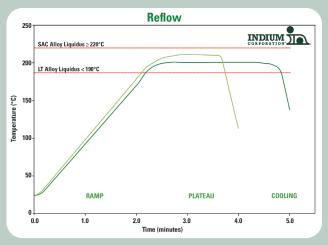
This profile is designed for use with **Durafuse**<sup>®</sup> **LT** (Indium10.2HFA). This can be used as a general guideline in establishing a reflow profile for **Durafuse**<sup>®</sup> **LT** Solder Paste. Deviations from these recommendations are acceptable, and may be necessary, based on specific process requirements.
