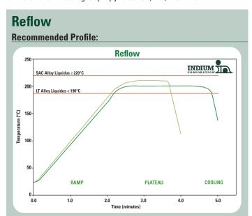
This profile is designed for use with **Durafuse® LT** (Indium10.2HFA). This can be used as a general guideline in establishing a reflow profile for **Durafuse® LT** Solder Paste. Deviations from these recommendations are acceptable, and may be necessary, based on specific process requirements.
