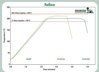
This profile is designed for use with **Durafuse**<sup>®</sup> LT (Indium10.8HFT). This can be used as a general guideline in establishing a reflow profile for **Durafuse**<sup>®</sup> LT Solder Paste. Deviations from these recommendations are acceptable, and may be necessary, based on specific process requirements.
