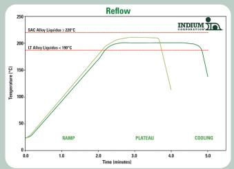
This profile is designed for use with **Durafuse**<sup>®</sup> LT (Indium10.8HFT). This can be used as a general guideline in establishing a reflow profile for **Durafuse**<sup>®</sup> LT Solder Paste. Deviations from these recommendations are acceptable, and may be necessary, based on specific process requirements.
