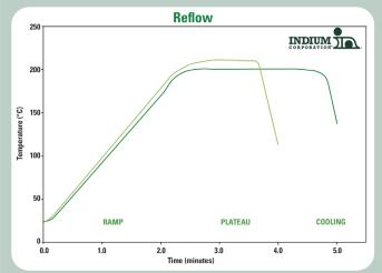
This profile is designed for use with **Durafuse**<sup>®</sup> **LT** (Indium3.2HF). This can be used as a general guideline in establishing a reflow profile for **Durafuse**<sup>®</sup> **LT** Solder Paste. Deviations from these recommendations are acceptable, and may be necessary, based on specific process requirements.
