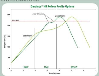
This can be used as a general guideline in establishing a reflow profile when using Durafuse® HR Solder Paste. Deviations from these recommendations are acceptable, and may be necessary. When selecting between the recommended linear and soak profiles, please take board size, thickness, and density into consideration. The flat soak portion of the linear profile (linear shoulder) may be eliminated.
