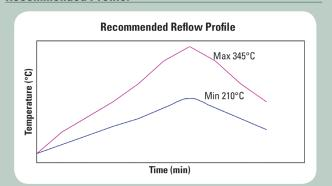
This is the standard reflow profile for **FC-WS-HT-A1**. The time to peak should be about 3 to 5 minutes. The peak temperature should be 20°C more than the melting point of the metal. Time above liquidus should be about 40 to 70 seconds.
