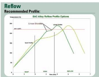
The stated profile recommendations apply to most Pb-free alloys in the Sn/Ag/Cu (SAC) alloy system, including SAC305 (96.5Sn/3.0Ag/0.5Cu). This can be used as a general guideline in establishing a reflow profile when using **Indium5.1ATR Solder Paste**. Deviations from these recommendations are acceptable, and may be necessary, based on specific process requirements, including board size, thickness, and density.
