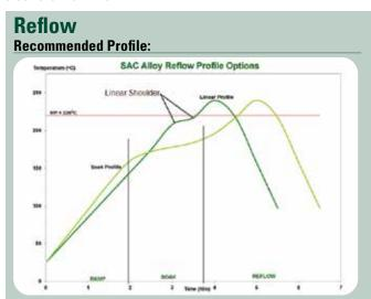
The stated profile recommendations apply to most Pb-free alloys in the SnAgCu (SAC) alloy system, including SAC305 (96.5Sn/3.0Ag/0.5Cu). This can be used as a general guideline in establishing a reflow profile when using **Indium5.8LS-4.5** solder paste. Deviations from these recommendations are acceptable, and may be necessary, based on specific process requirements, including board size, thickness, and density.
