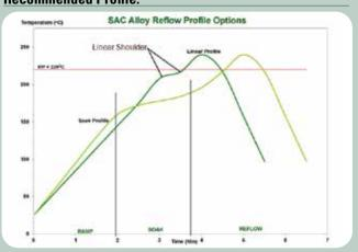
The stated profile recommendations apply to most Pb-free alloys in the SnAgCu (SAC) alloy system, including SAC305 (96.5Sn/3.0Ag/0.5Cu). This can be used as a general guideline in establishing a reflow profile when using **Indium5.8LS-4.5** solder paste. Deviations from these recommendations are acceptable, and may be necessary, based on specific process requirements, including board size, thickness, and density.
