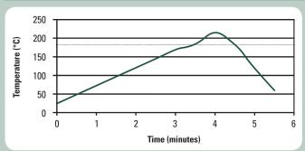
The profile shown here is designed for **Indium6.3** with Sn63/Pb37 and Sn62/Pb36/Ag2 under both air and nitrogen reflow atmosphere. It serves as a general guideline in establishing a reflow profile for these alloys.
