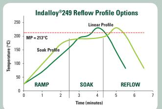
The stated profile recommendations can be used as a general guideline in establishing a reflow profile when using **Indium8.9HFC Solder Paste**. Deviations from these recommendations are acceptable, and may be necessary, based on specific process requirements, including board size, thickness, and density. Start with the linear profile, then move to the optional soak profile, if needed. The flat soak portion of the linear profile (linear shoulder) may also be eliminated.
