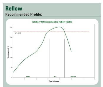
This can be used as a general guideline in establishing a reflow profile when using Indium8.9HFRV with Indalloy®292 Solder Paste. Deviations from these recommendations are acceptable, and may be necessary, based on specific process requirements, including board size, thickness, and density. Start with the linear profile. If needed, a flat soak portion or linear shoulder may be added to reduce the thermal gradient.
