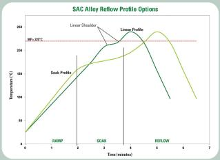
The stated profile recommendations apply to most Pb-free alloys in the SnAgCu (SAC) alloy system, including SAC305 and SnAgCuSb. This can be used as a general guideline in establishing a reflow profile when using **Indium8.9HFRV Solder Paste**. Deviations from these recommendations are acceptable, and may be necessary, based on specific process requirements, including board size, thickness, and density. Start with the linear profile, then move to the optional soak profile, if needed.
