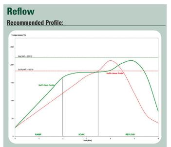
This profile is designed for use with Sn63/Pb37 and Sn62/Pb36/Ag2 and can serve as a general guideline in establishing a reflow profile for use with other alloys. Adjustments to this profile may be necessary based on specific process requirements. Start with the linear profile, then move to the optional soak profile, if needed.
