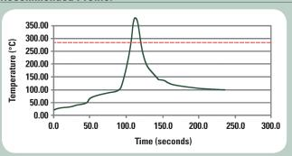
The typical profile above is designed for use with high-Pb (lead content 80% or greater) alloys in a forming gas or nitrogen atmosphere. This profile can serve as a general guideline for establishing a profile for your process and should be regarded as a typical example. Adjustments to this profile may be necessary based on assembly size, thermal density, and other factors. Use of other alloys with lower or higher liquidus temperatures will also require changes.
