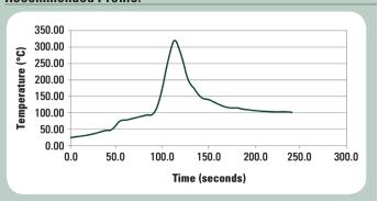
The typical profile above is designed for use with Sn10/Pb88/Ag2 or Sn5.0/Pb92.5/Ag2.5 alloy in a forming gas or nitrogen atmosphere (100ppm oxygen or less). It can serve as a general guideline for establishing a profile for your process and should be regarded as a typical example. Adjustments to this profile may be necessary based on assembly size, thermal density, and other factors. Use of other alloys with lower or higher liquidus temperatures will also require changes.
