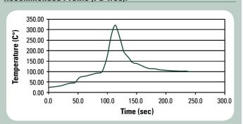
The typical profile above is designed for use with high-Pb (lead content 80% or greater) alloy in a forming gas or nitrogen atmosphere (100ppm oxygen or less). It can serve as a general guideline for establishing a profile for your process and should be regarded as a typical example. Adjustments to this profile may be necessary based on assembly size, thermal density, and other factors. Use of other alloys with lower or higher liquidus temperatures will also require changes.
