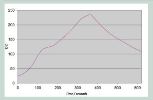
Flip-Chip Flux NC-26S is intended to be used in a nitrogen reflow environment of 100ppm oxygen or less. Some applications can utilize this material in an air environment, although best results will be obtained in an inert atmosphere. Flip-Chip Flux NC-26S can be used on many surface finishes including immersion Ag, Cu, and AuNi. These surfaces can be soldered with Pb-free alloys, but require nitrogen if reflow temperatures exceed 240°C.
