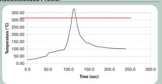
The typical profile above is designed for use with high-Pb (lead content 80% or greater) alloys in a forming gas or nitrogen atmosphere (100ppm oxygen or less). This profile can serve as a general guideline for establishing a profile for your process and should be regarded as a typical example. Adjustments to this profile may be necessary based on assembly size, thermal density, and other factors. Use of other alloys with lower or higher liquidus temperatures will also require changes.
