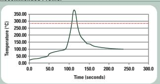
The typical profile above is designed for use with high-Pb (lead content 80% or greater) alloys in a forming gas or nitrogen atmosphere. This profile can serve as a general guideline for establishing a profile for your process and should be regarded as a typical example. Adjustments to this profile may be necessary based on assembly size, thermal density, and other factors. Use of other alloys with lower or higher liquidus temperatures will also require changes.
