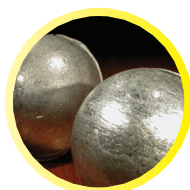
Cadmium Increases corrosion resistance of solders. Increases service temperature and strength of solder. Used in electroplating and fission rate control in nuclear reactors.
