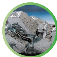
When alloyed with indium, creates an alloy that is liquid at room temperature and used in thermal applications. Low-temperature metal enables flexible/self-healing circuits and soft robotics.
