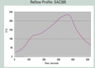
A short preheat (150°-160°C) for less than 45 seconds may be used to reduce voiding. The profile should ideally be a linear ramp at 2-3°C/second up to 20-30°C above solidus temperature, with a slow cool down afterwards of -0.5 to -0.2°C, and a minimum time above liquidus of 60 seconds.
