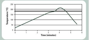
Peak reflow temperature should be <350°C in a nitrogen atmosphere (<50ppm  $O_2$ ), with a linear ramp up to 30°C above liquidus. These profiles are recommended to the user as starting points, and should be optimized by the user to meet their individual process needs.
