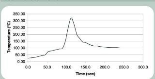
The typical profile above is designed for use with alloys containing greater than 84% lead (Pb) in a forming gas or nitrogen atmosphere. It can serve as a general guideline for establishing a profile for your process and should be regarded as a typical example. Adjustments to this profile may be necessary based on assembly size, thermal density, and other factors. Use of other alloys with lower or higher liquidus temperatures will also require changes.
