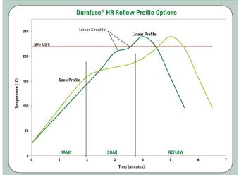
This can be used as a general guideline in establishing a reflow profile when using **Durafuse® HR Solder Paste**. Deviations from these recommendations are acceptable, and may be necessary. When selecting between the recommended linear and soak profiles, please take board size, thickness, and density into consideration. The flat soak portion of the linear profile (linear shoulder) may be eliminated.
