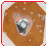
Typical Spatter 10.3% Spatter
