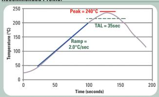
**SiPaste® C312HF** should be reflowed using a linear profile in a nitrogen atmosphere. The stated profile recommendations can be used as a general guideline in establishing a reflow profile for **SiPaste® C312HF** with SnAgCu, SnAg, and SnSb alloy systems.
