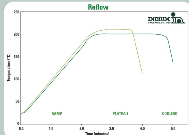
This profile is designed for use with Durafuse® LT (Indium12.9HF). This can be used as a general guideline in establishing a reflow profile for Durafuse® LT Solder Paste. Deviations from these recommendations are acceptable, and may be necessary, based on specific process requirements.
